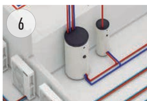
Buffer Tank of 1.000L.
