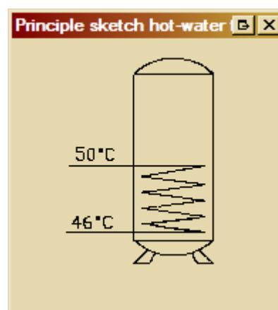
**Fig. 20: Principle sketch of a sanitary tank with good layering and low mixing of water temperatures**
