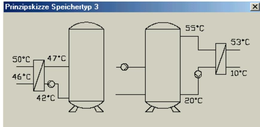
Fig. 22: principle sketch for different tanks, type 3
