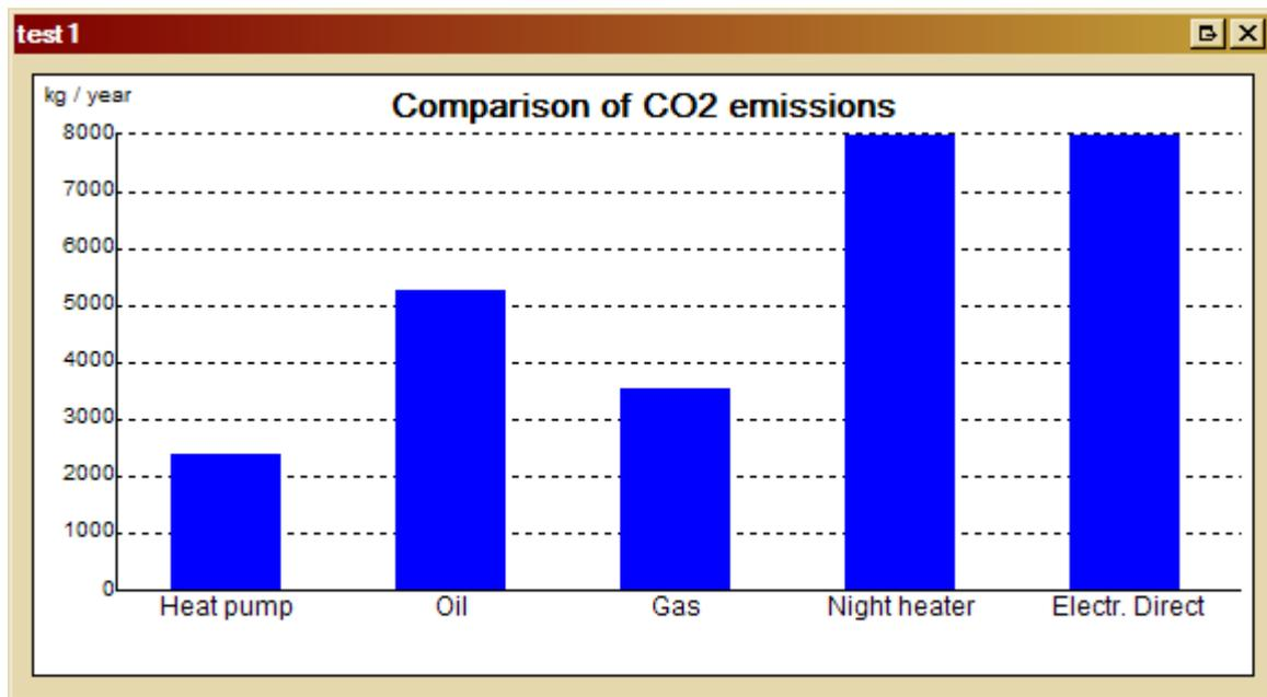
Fig. 50: Comparison of CO<sub>2</sub>-emissions in the current project
