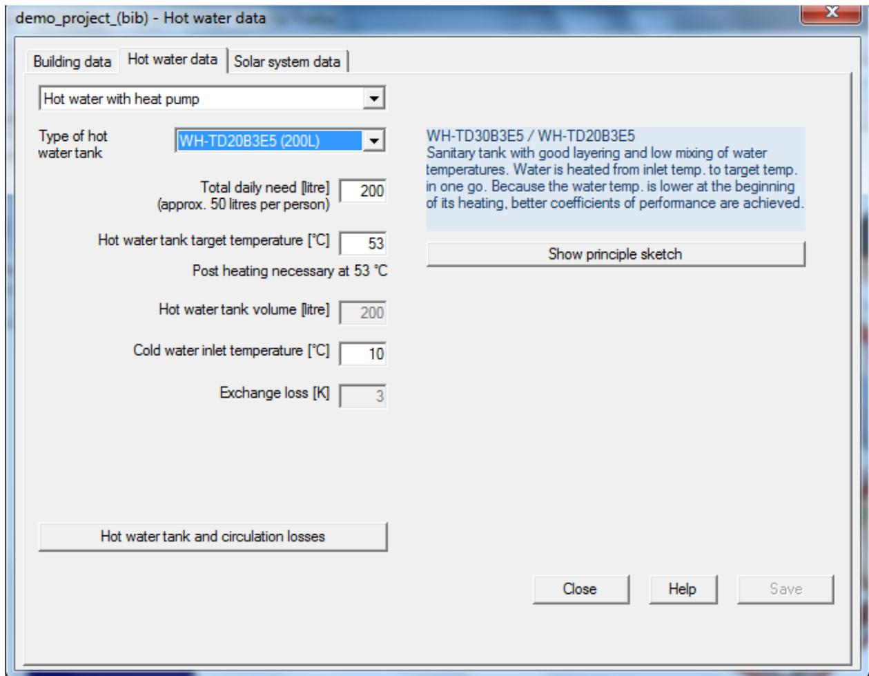
**Fig. 7: Choice of a tank at “Hot water data” sheet (Quick design)**
