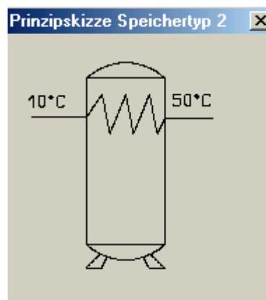
**Fig. 21: Sketch of a tank with bad layering, type 2**
