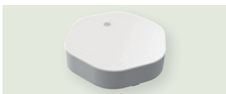
Water leakage sensor. Two sensing pads under the body activate when water is present between the two pads. Detecting the water, the sensor reports the event to the controller (and BEMS).
