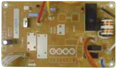
CZ-NS2P PCB for solar connection kit for Mono-bloc systems.
