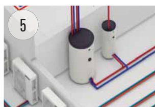
Buffer Tank of 1000L.
