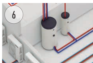
Buffer Tank of 1.000L.
