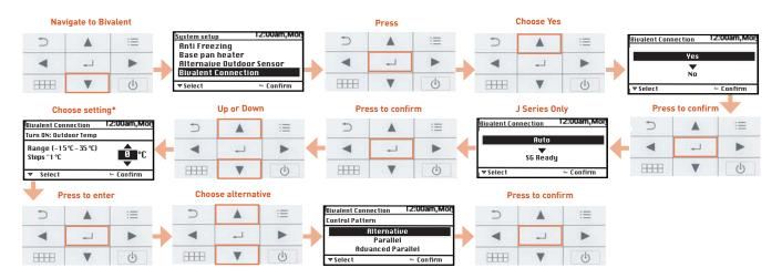
\* "Turn On" set point: This is the setting at which the outside temperature must be at or below before bivalent operation starts.
