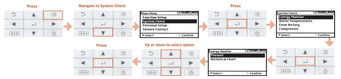
b) Water Temperatures: Shows current outlet/inlet etc temperatures.
