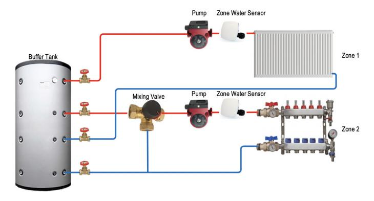
The system needs to know the flow temperature of circuit in order to make adjustments. This is why the zone water sensors are needed.
