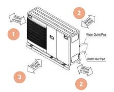
Clearance around unit required for operation. For Single & Twin fan units:
