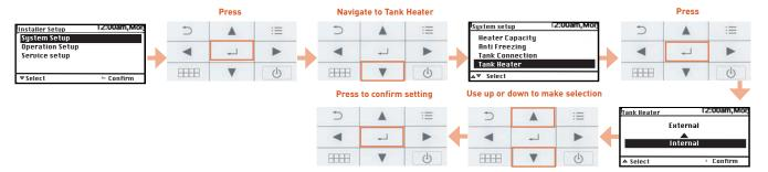
When set to "External, "Tank heater ON time" must be set. This is the delay time that the system will wait, after beginning a DHW cycle, before automatically engaging the booster heater.
