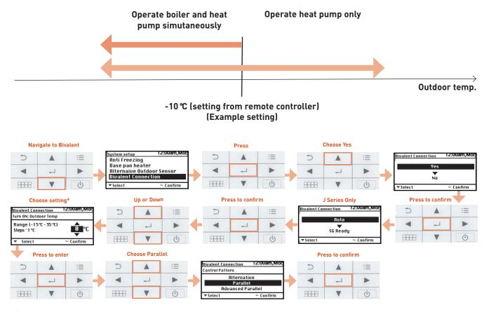
\* "Turn On" set point: This is the setting at which the outside temperature must be at or below before bivalent operation starts.
