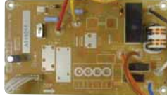
CZ-NS3P PCB for solar connection kit for Mono-bloc systems 6kW and 9kW.
