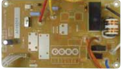
CZ-NS2P PCB for solar connection kit for Mono-bloc systems.
