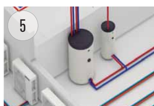
Buffer Tank of 1000L.
