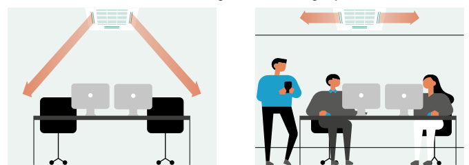
Circulation by detecting no movement (10 minutes).
