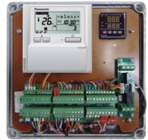
PCB, Transformer, Solenoid Control Valve, Thermistor x 4 pcs, Terminal Base and Electrical Component Box.
