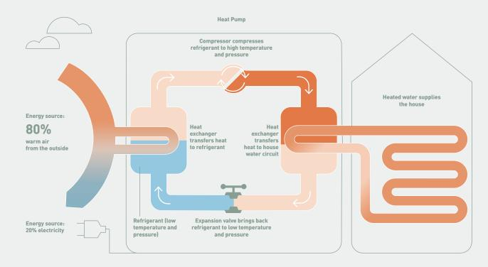
With Aquarea, up to 80% of the heat energy required is taken from the ambient air. Aquarea captures latent heat energy from the ambient air and transfers it to heat the water needed to warm your home or for domestic hot water and even to cool the house if required.
