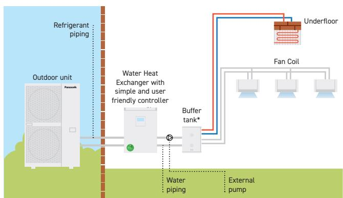
\* Minimum buffer tank volume: 10 L/kW. \*\* Diagram is for illustrative purpose only.
