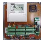
PCB, Power trans, Terminal block
