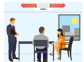
Indirect air flow by detecting movement
