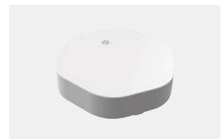
Water leakage sensor. Two sensing pads under the body activate when water is present between the two pads. Detecting the water, the sensor reports the event to the controller (and BMS).
